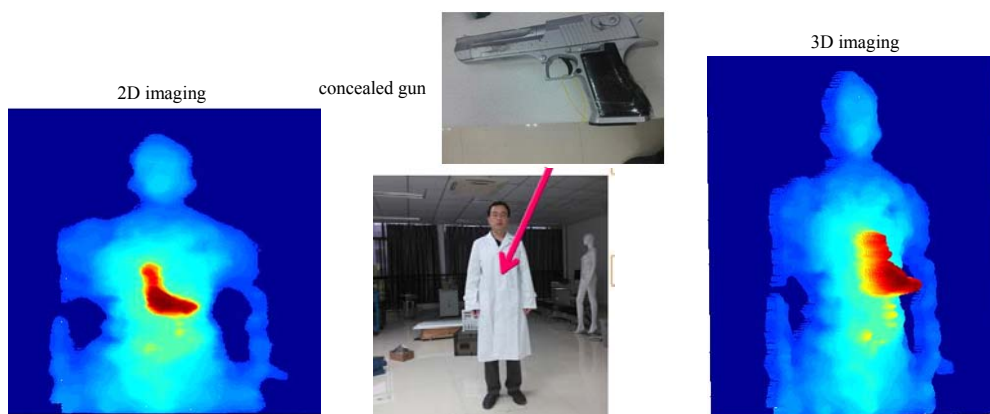
Fig.6 Radar image of a person with a concealed gun 图 6 人体隐藏危险品雷达成像结果
