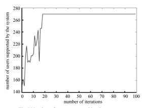
Fig. 5 Number of users supported by the system vs. the number of iterations
