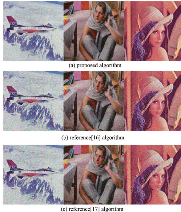
Fig.10 Test results of three algorithms against noise attack ( K=0.1 ) 图 10 3 种算法的抗噪声攻击测试结果( K=0.1 )
