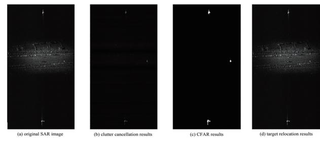
Fig.3 STAP-GMTI results of typical frames 图 3 典型动目标检测结果
