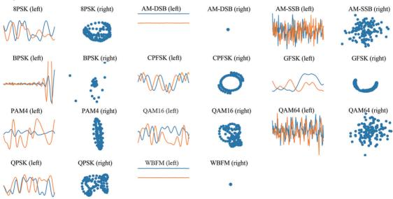
Fig.1 Time domain distribution (left) and constellation (right) of different modulated signals 图 1 不同调制信号时域分布图(left)和星座图(right)
