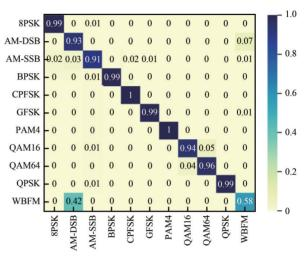
Fig.5 Recognition rate confusion matrix of this mode at 14 dB 图 5 本文模型在 14 dB下识别率混淆矩阵
