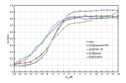
Fig.6 Recognition rate of each model under different SNRs 图 6 不同信噪比下各模型识别率
