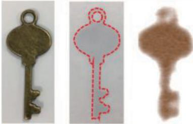
Fig.14 Terahertz(0.3 THz) imaging based on  $\text{Ir}_{0.7}\text{Pt}_{0.3}\text{Te}_2$  material
