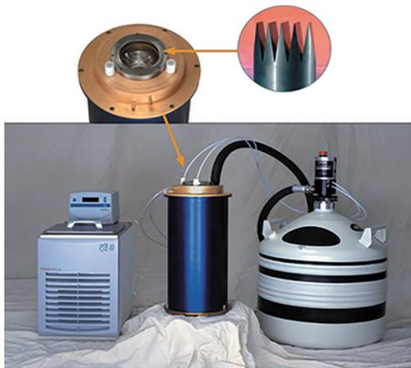
Fig.9 NBS-400 primary noise standard produced by Noisecom in USA
