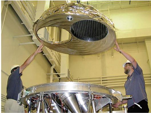
Fig.7 3~90 GHz blackbody radiation source of NASA
