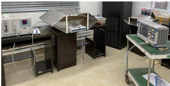
Fig.7 Transient magnetic field measurement system
