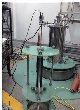
Fig.10 Testing system for sensitivity coefficient of transient magnetic field sensor
