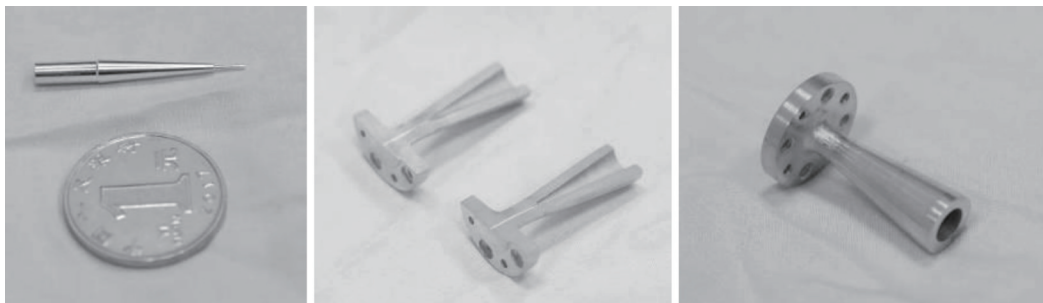
Fig.10 Electroforming mandrel and product of 425 GHz feed horn 图10 425 GHz 高频馈源喇叭电铸芯模、馈源喇叭实物
