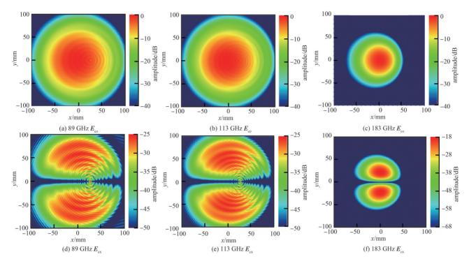
Fig.7 Normalized electric field contour of near-field for each frequency channel 图 7 各频率通道近场的归一化电场等高图
