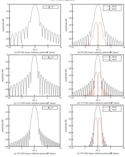
Fig.6 Far-field normalized radiation pattern of each frequency channel 图 6 各频率通道的远场归一化辐射方向图
