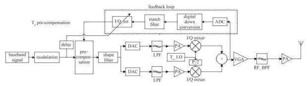
Fig.3 Block diagram of unbalanced pre-compensation for I/Q at the transmitter 图 3 发端 I/Q 不平衡预补偿框图
