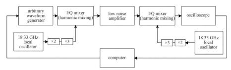
Fig.7 Diagram of I/Q unbalanced experimental link 图 7 I/Q不平衡实验链路图
