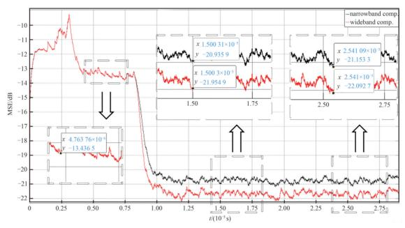
Fig.11 Comparison chart of MSE for measured I/Q imbalance wide and narrow band algorithms 图 11 实测 I/Q 不平衡宽窄带算法 MSE 对比图
