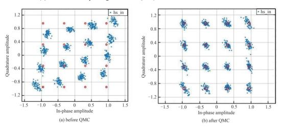
Fig.9 Constellation before and after calibration 图 9 校正前后星座图
