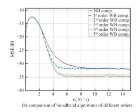
Fig.6 Comparison chart of MSE for I/Q imbalance algorithms 图 6 I/Q不平衡算法 MSE对比图
