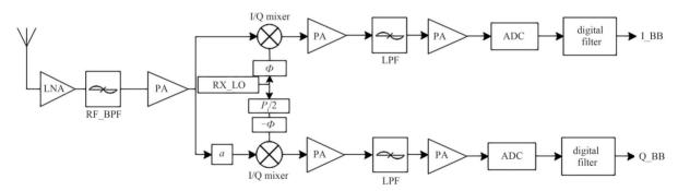
Fig.1 Block diagram of narrowband signal I/Q imbalance receiver 图 1 窄带信号 I/Q 不平衡接收机框图
