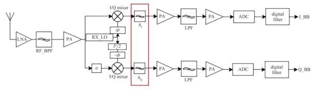
Fig.2 Block diagram of wideband signal I/Q imbalance receiver 图 2 宽带信号 I/Q 不平衡接收机框图
