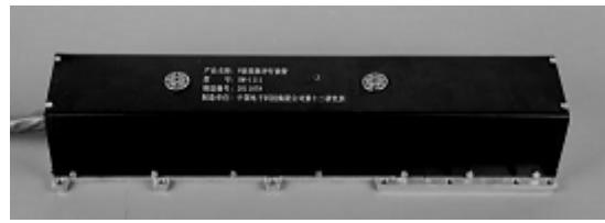
Fig.2 Photo of W band pulsed TWT for THz TWT cascade multiplier
