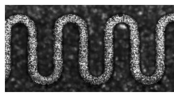
Fig.7 Photo of 2nd harmonic folded waveguide SWS
