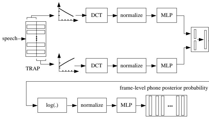
Fig.3 Architecture of detecting phone posterior probability
