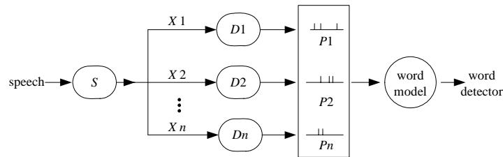
Fig.1 Architecture of keywords spotting framework
