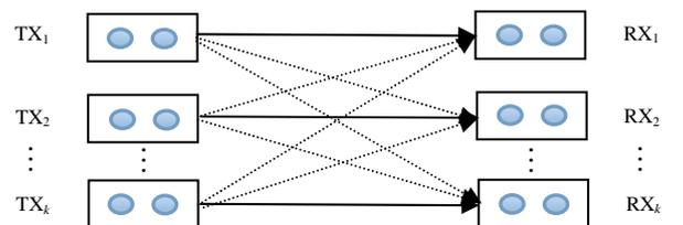
Fig.1 The  $k$ -user MIMO interference channel. Transmitter  $k$ , with  $M_k$  antennas, has a message for receiver 1 with  $N_1$  antennas. All transmitters share a channel with all receivers
