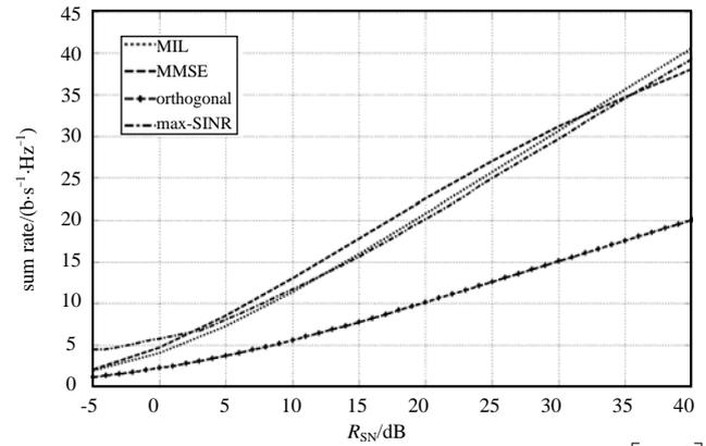
Fig.2 Sum rate performance of the 3 algorithms:  $K=3$ ,  $N_k=M_k=2$ ,  $E[\|X_k\|^2]=1$
