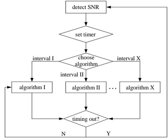
Fig.3 Flow chart of the proposed adaptive selection mechanism
