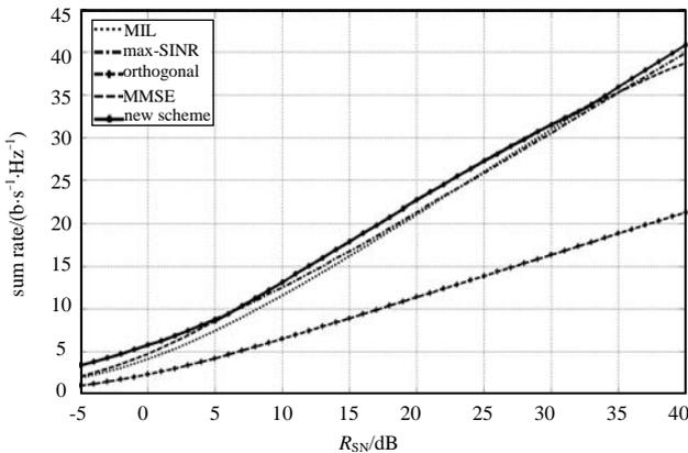
Fig.4 Sum rate performance of the proposed adaptive selection mechanism:
