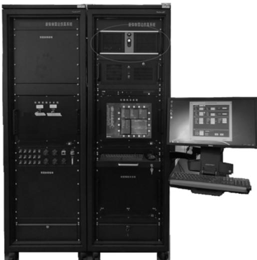
Fig.5 Real-time SAR/ISAR imaging system
