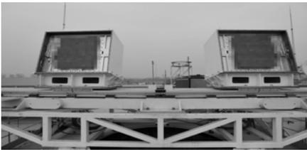
Fig.4 Prototype of C band monopulse radar
