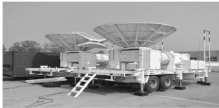
Fig.5 Prototype of C band phased array radar
